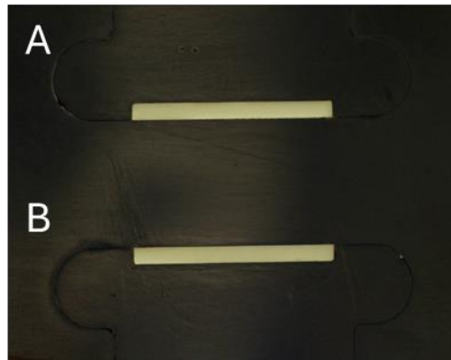
Figura 3. Barras de comopiste; A. Grupo 1C (BFFRW): Barra de resina 3M™ FILTEK™ BULK FILL FLOWABLE RESTORATIVE+ Ribbond THM, Ribbond Inc, Seattle, WA, EE. UU.) + Ribbond Wetting resin ; B. Grupo 2C (EFRW): Barra de resina everX Flow (GC, Tokyo, Japan) + Ribbond THM, Ribbond Inc, Seattle, WA, EE. UU.)+ Ribbond Wetting resin.
