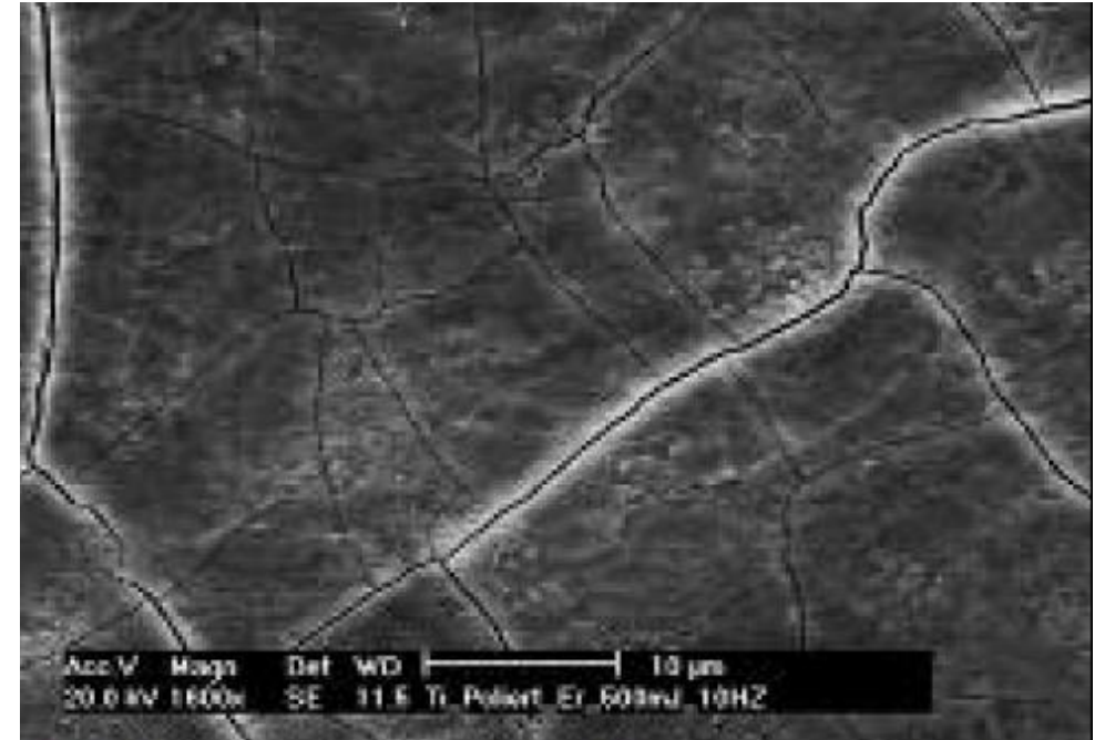
Fig 5 Typical cracks on polished titanium surface after 10 seconds of irradiation with the Er:YAG laser (500 mJ/10 Hz).
