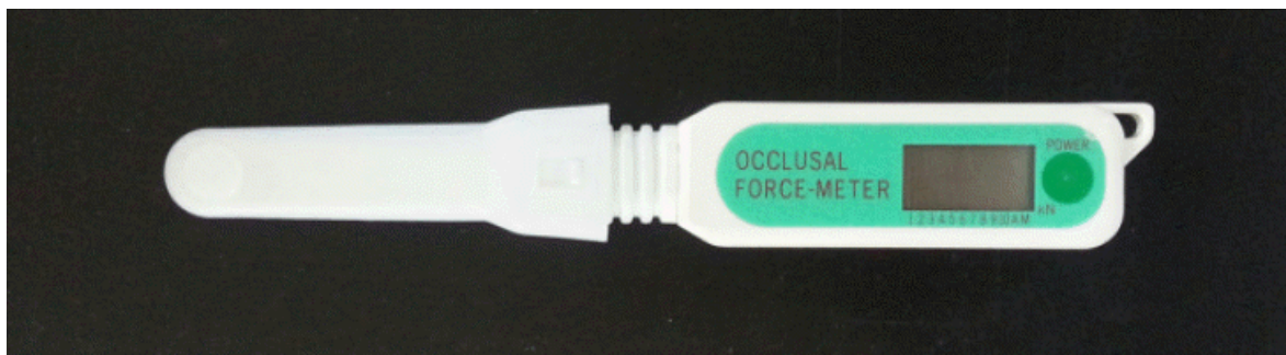
Figura 1. Gnatodinamometro - Occlusal Meter GM10 Nagano Keiki
