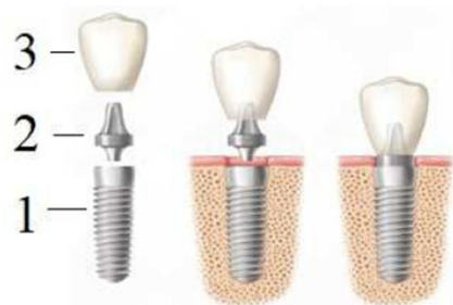
Figure 5. Dental prosthesis: 1—implant, 2—abutment, 3—crown.
